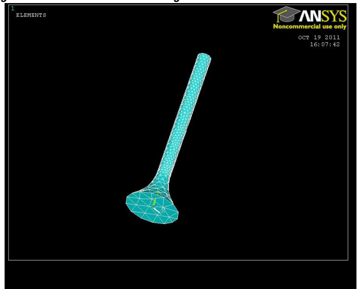
Fig.7: Free Tetra meshing for small sized exhaust valve (2 cm)
